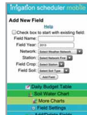
Add New Field page: Name field, select station and define field variables.
